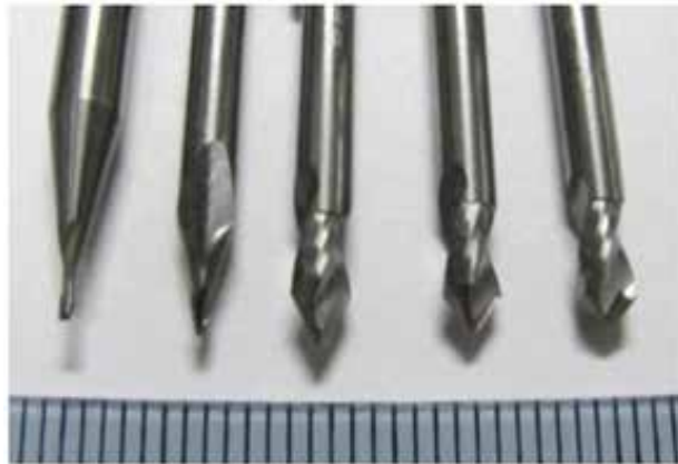
Fig.3: Micro-milling tools(from left to right): straight tool, 150, 300, 400 and 500 tapered tools. [12]
