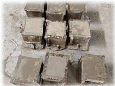
Fig. 1. Casting of cubes
