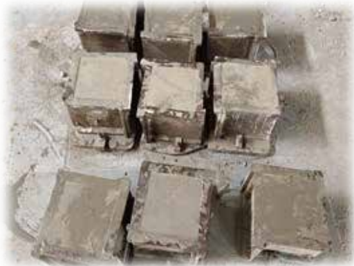
Fig. 1. Casting of cubes
