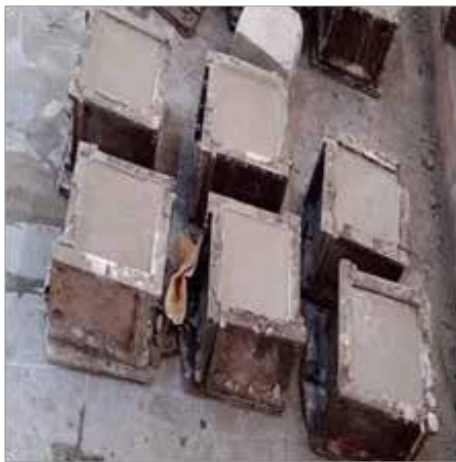
Fig.2. Casting of blocks
